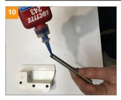
Now prepare the Turtle for installation. The threaded To tighten a threaded rod in a hole, place two nuts rod must first be secured in the Turtle, using thread lock and two M10 nuts.
