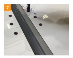
The holes must be drilled out to 16 mm on the inside of the door. This should NOT be drilled through. It should be drilled to the other side, but not through. DRILL CAREFULLY! (This applies to all 6 holes.)
