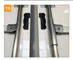
Rubbers are inserted between the Turtle and the door. These are also used to raise the height of the lock to the same height. The doors will not always close flush. There is almost always a door that lies lower than the other door.
