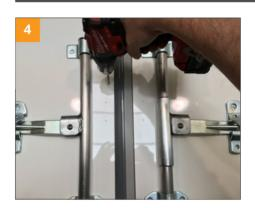
There are 6 points on the template where holes have to be drilled.
